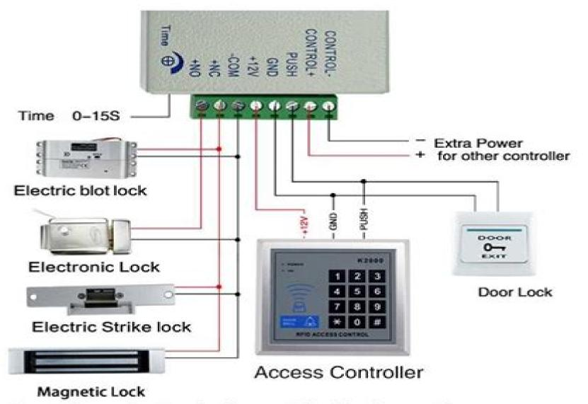
Attention when electronically contriled lock must be transferred to 0seconds delay, to prevent burning of electric lock.
