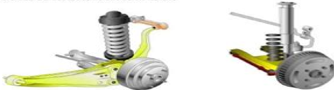
Left: Multi-link rear suspension. This design has two lower control arms. Right: Modified MacPherson strut rear suspension. Note the tie rod end bolted to the control arm, used to adjust rear toe.
