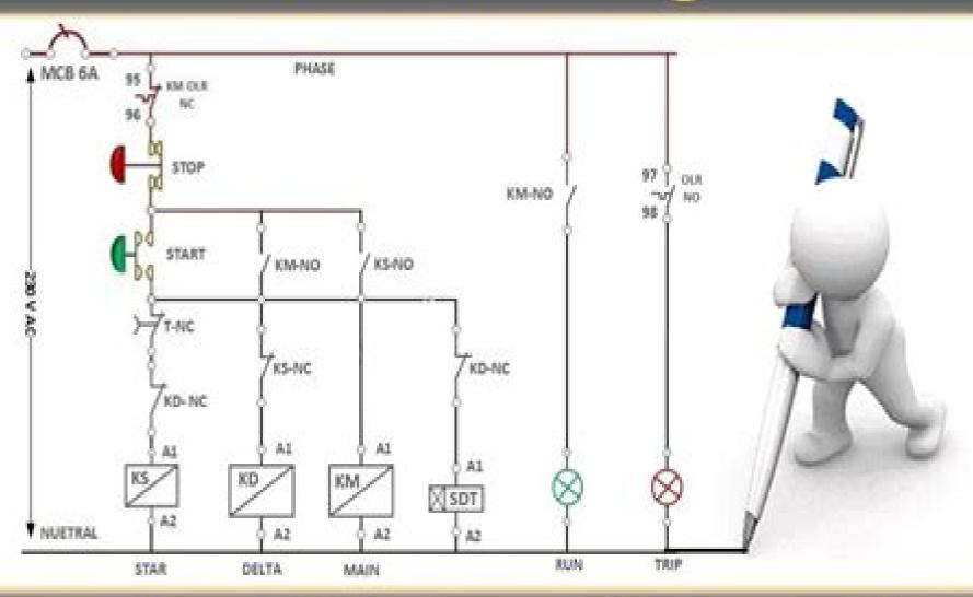
**Control Panel Wiring | Star Delta Power Wiring**
