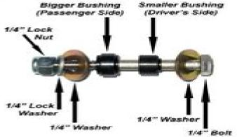
18. Take the 2 provided steel bushings and place them on each side of the shift fork. The bigger one goes on the passenger side. Please note that the shoulders enter into the shift fork holes and they can be held in place on the shift fork by greasing them generously.
