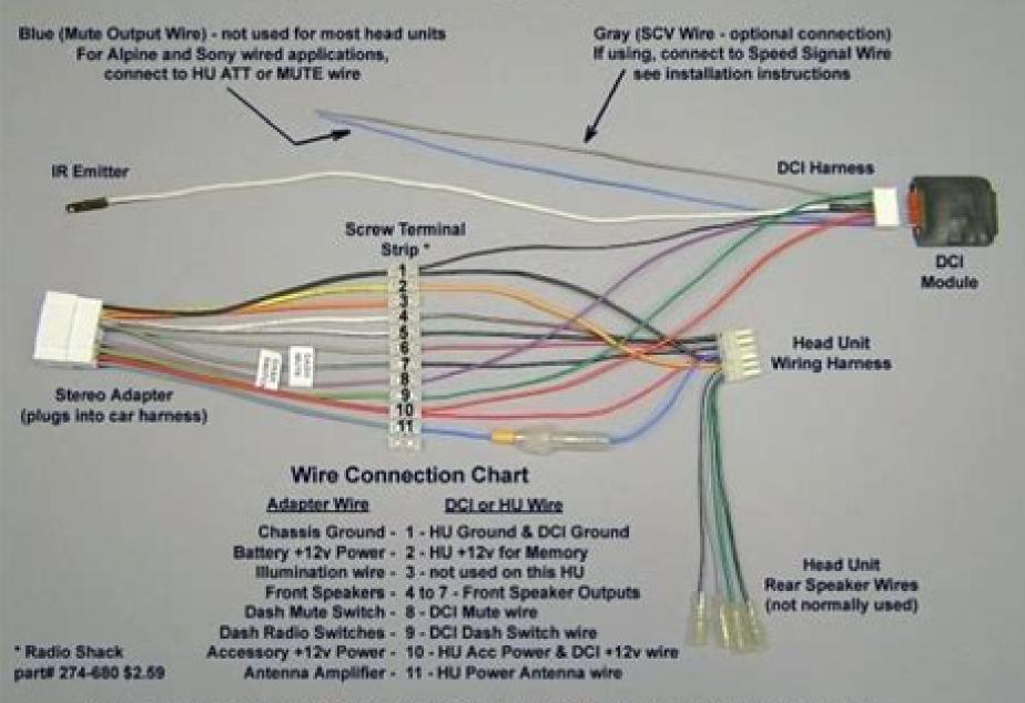
Note: This drawing shows an IR DCI, but the wiring is similar for all types of DCI's. Different HU brands may have different wire colors on the HU Wire Harness, so check your head unit manual before wiring.
