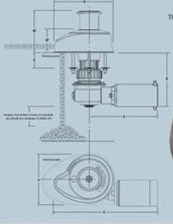
The Freedom Series of automatic rope/chain anchor winches incorporate Maxwell's latest design technology for rope to chain spliced rodes.
