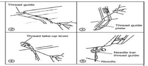
Raise the thread take-up lever to its highest position by turning the handwheel toward you. Raise the presser foot.
