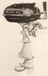
ALTERNATE FIRING TWIN 7.2 H. P. 44 LBS. (Approx.) CERTIFIED AT 4000 R.P.M.
