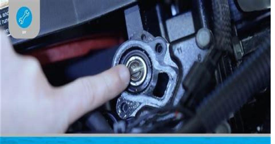
HOW TO INSPECT AND CHANGE THE THERMOSTAT IN A MERCURY 40-60HP FOURSTROKE
