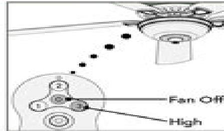
Within 3 minutes of restoring power to the fan, press both the **FAN OFF** button and the **HIGH** button for at least 4 seconds.
