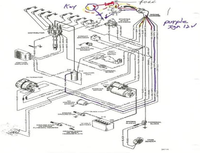
MCM 200 5.0 Litre Engine (Battery Meter Circuit)
