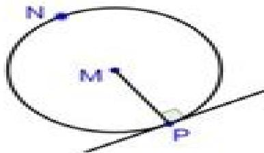
A radius is perpendicular to a tangent at the point of tangency.
