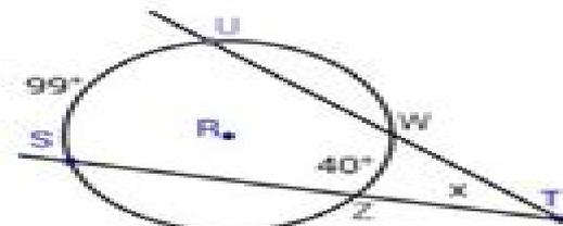
An angle formed by two secants is one-half the difference of its intercepted arcs.
