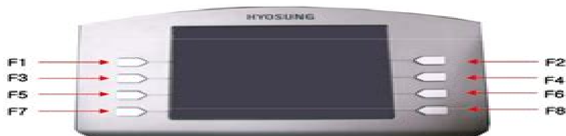
- Function Key Location on ATM -
