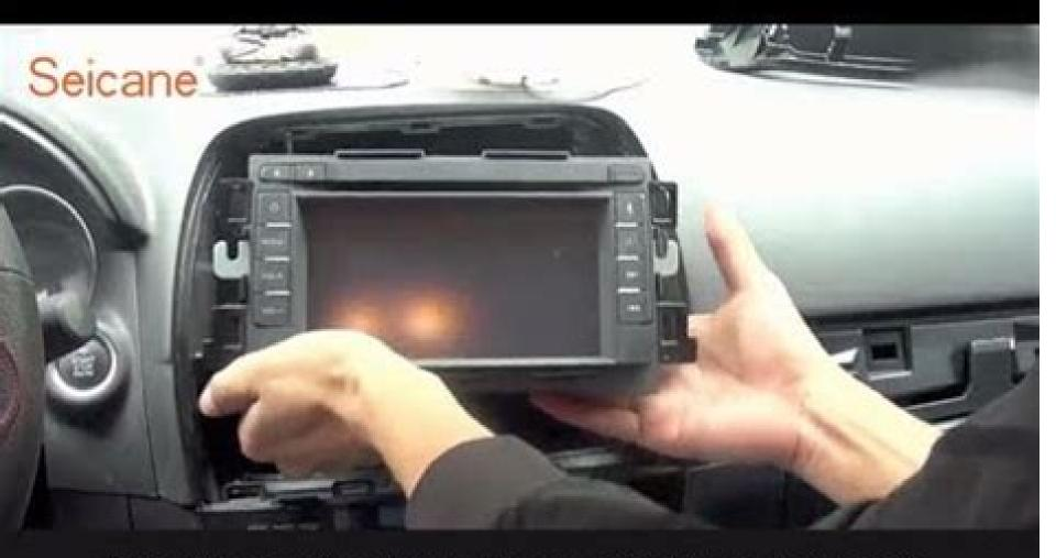
Take out the car radio and unplug the connectors at the back of the radio
