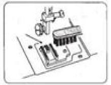
With a brush, clean out dust and line clogged on the feed dog teeth. Reset the needle plate.
