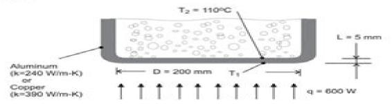
ASSUMPTIONS: (1) One-dimensional, steady-state conduction through bottom of pan.
