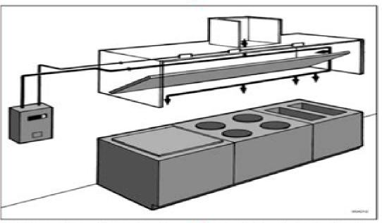
The detection portion of the fire suppression system allows for automatic detection by means of specific alloy rated fusible links, which, when the temperature exceeds the rating of the link, the link separates, allowing the regulated release to actuate.
