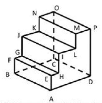
Fig 13b Isometric View (Hidden details)
