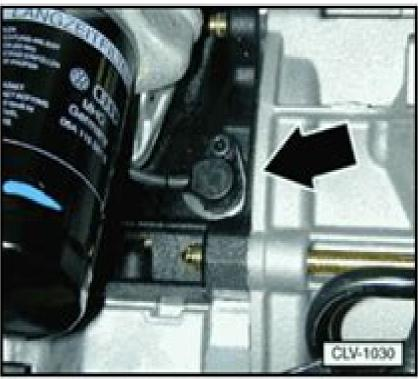
G28 Engine Speed (RPM) sensor (2.0 ltr. engine)
