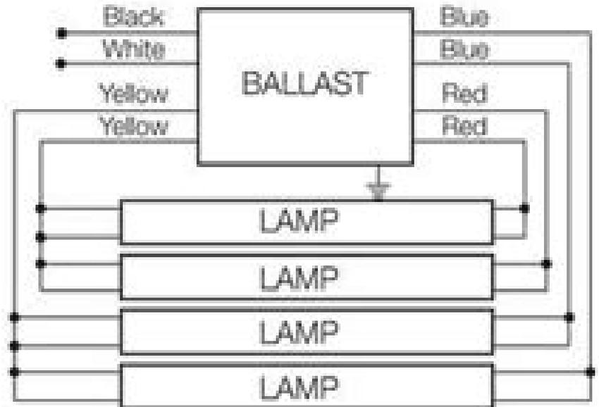
Note: For three lamp application, cap any unused blue lead. Insulate to 600 volts.
