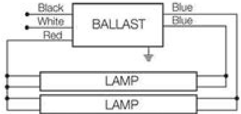
Note: For one lamp application, cap any blue lead. Insulate to 600 volts.
