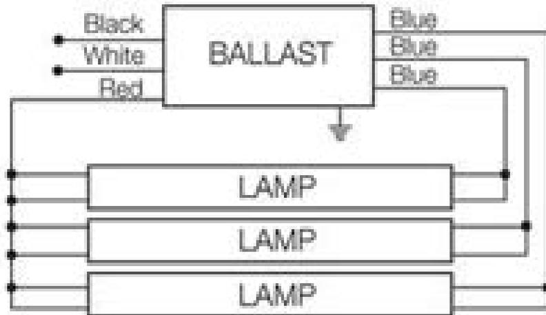
Note: For two lamp application, cap any blue lead. Insulate to 600 volts.
