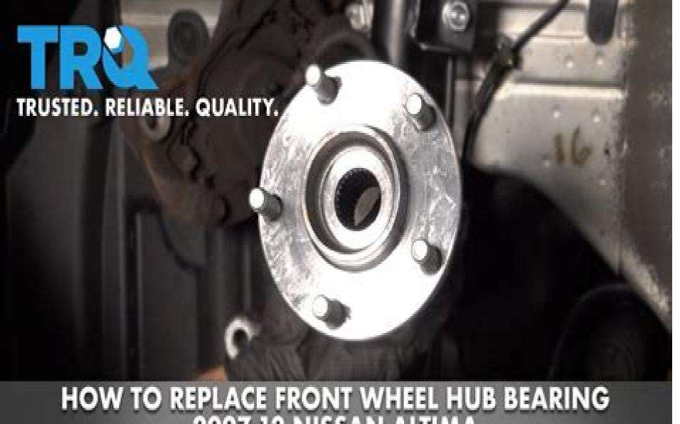
HOW TO REPLACE FRONT WHEEL HUB BEARING 2007-12 NISSAN ALTIMA
