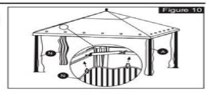
From inside the gazebo, attach the insect panel net (L) to the rod on the inside of the crossbars with using the Velcro<sup>®</sup> tabs. See Figure 11.
