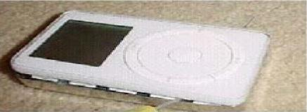
Use your flat tool to gently pry the casing up all along these notches to release the plastic casing from the metal pan.
