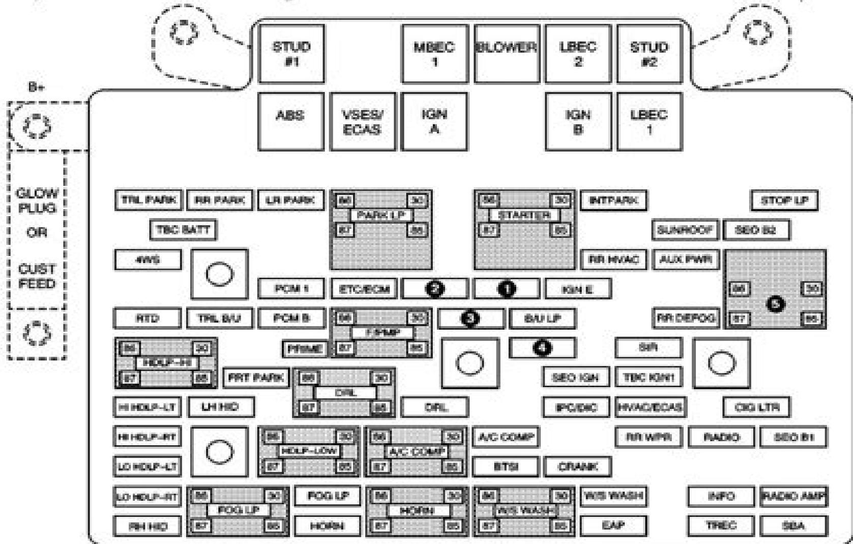
\* NOTE: The function and amperage of these fuses are different for gas and diesel fueled engines. See Owners Manual
