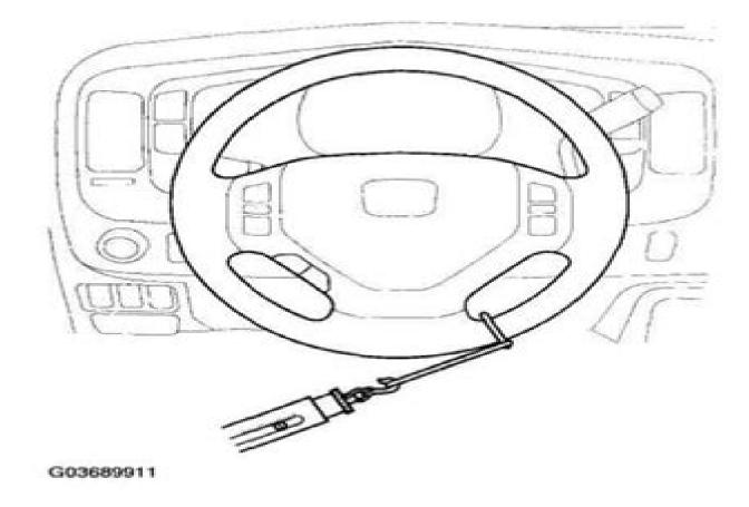
Fig. 4: Checking Power Steering Initial Turning Load Courtesy of AMERICAN HONDA MOTOR CO., INC.
