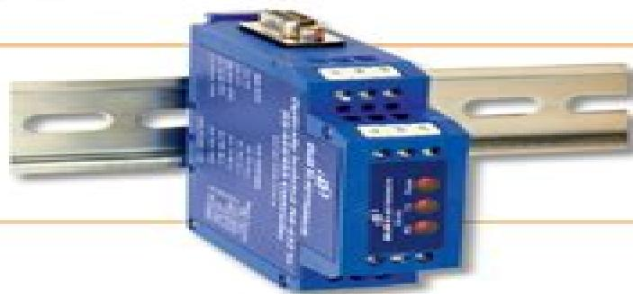
The 485LDRC9 is an optically isolated RS-232 to RS-422/485 converter. RS-232 signals interface through a DB9 female connector or a terminal block. RS-422/485 signals and power inputs connect to the terminal block. Terminal blocks are arranged to allow easy wiring inside a control panel.
