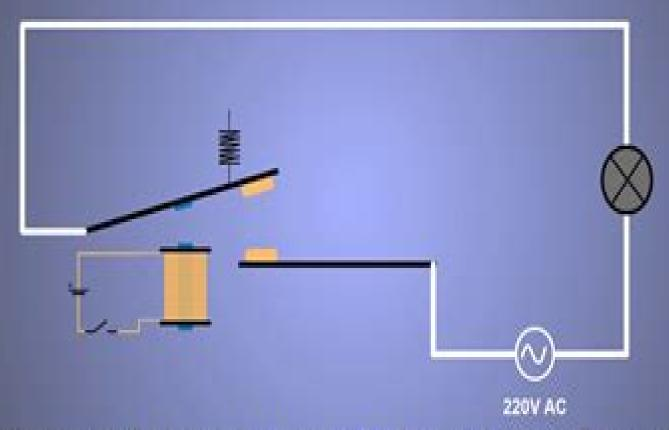
When the control switch is turned ON current starts flowing through a coil, it generates magnetic field that
