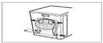
2. Unscrew the 4 bolts with the wrench supplied.
