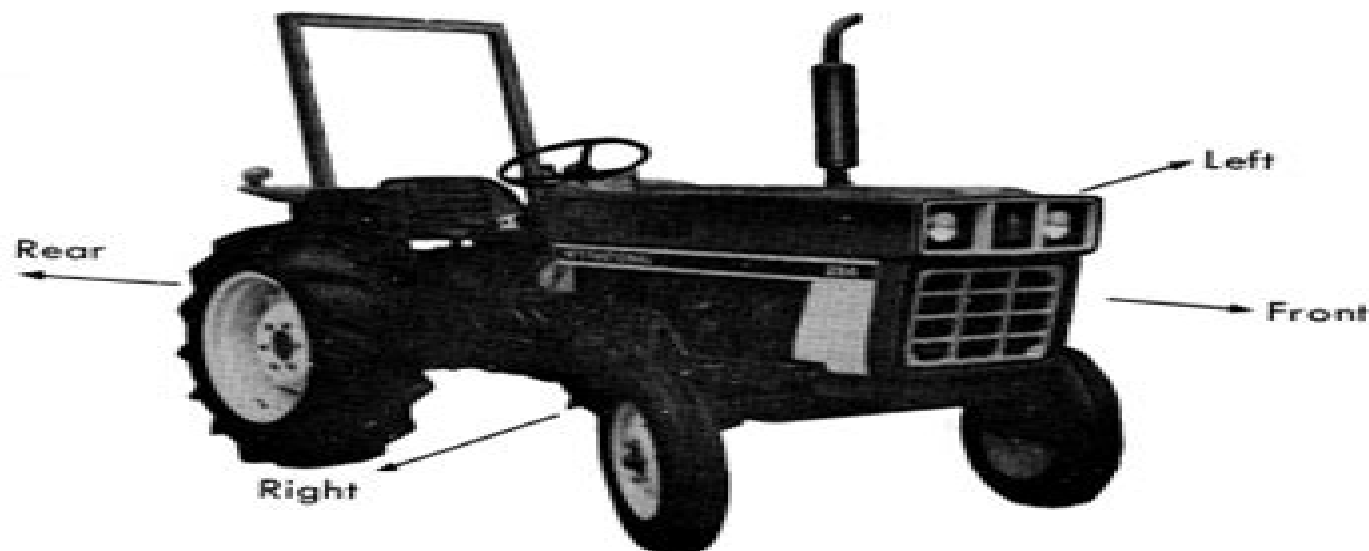
International 284 Tractor showing terms of location (Tractor in picture with operator protective frame)
