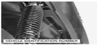
The registered number plate is attached on the left side of the frame near the rear shock absorber.
