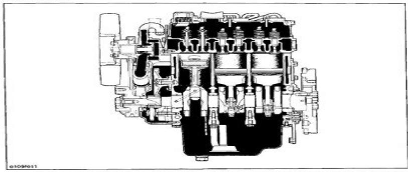
The D662-L, D662 and D722 are vertical, liquid cooled, 4-cycle diesel engines, utilizing Kubota's unique combustion system "NTVCS", special designed engine, the well-known Bosch MD type injection pump, alminum radiator for greater heat
