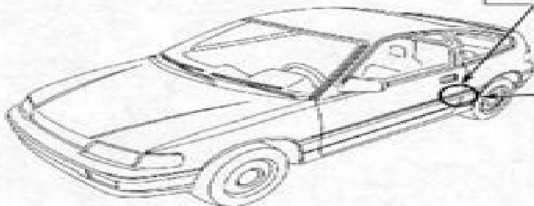
**Vehicle Identification Number and Federal Motor Vehicle Safety Standard Certification**
