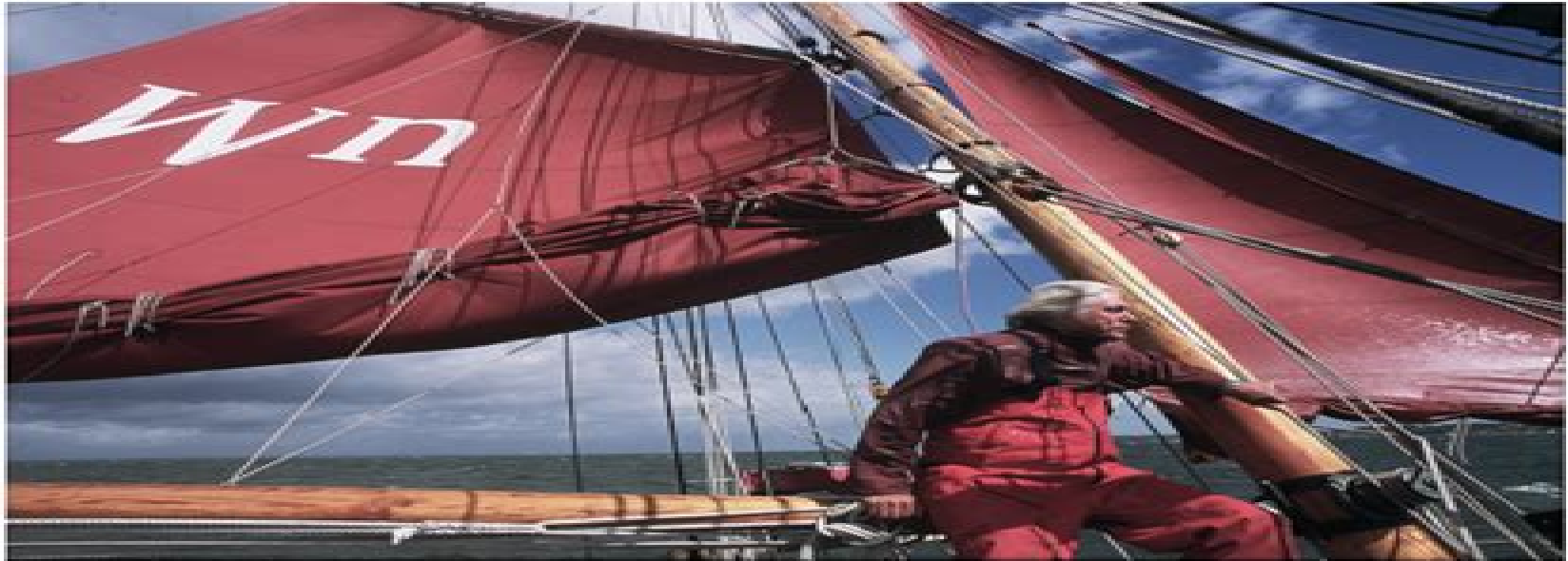
Tom on board Westernman with the main triced up. Gaff rig is supremely flexible for sail area and balance
