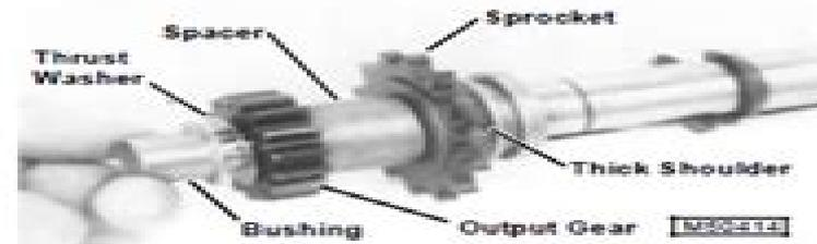
11. Install reverse sprocket with thicker shoulder toward shifter collar.
