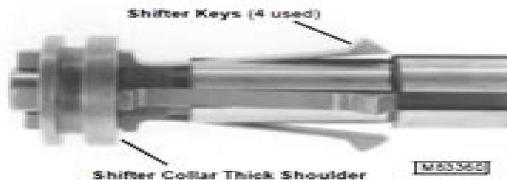
10. Position keys in keyways near end of shifter shaft and hold in place with heavy rubber band or plastic tie strap that can be cut when finished. Install shifter collar over key tabs with thicker shoulder of collar toward center of shaft. Slide collar and keys onto center of shaft.
