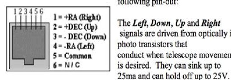
The Left, Down, Up and Right signals are driven from optically isolated photo transistors that conduct when telescope movement is desired. They can sink up to
