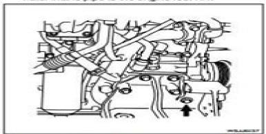
Remove the bolt with arrow mark which holds the blow-by hose to the engine foot RH.
