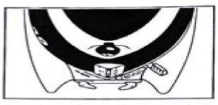
The Twist-Shift mechanism is so designed that the mater will not shift when the speed indicator lever is to the right of the red "shift" line on the decal.
