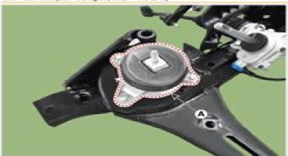
3. Remove the LH engine mounting support bracket (A).
