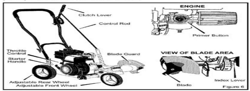
Throttle Control - Controls the engine speed.
