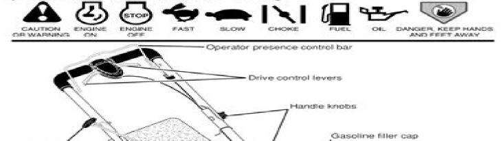
cascher Air filter Engine oil cap with dipstick Muttler
