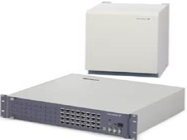
The BusinessPhone communication system offers large-system capabilities in a package that is cost-effective for small and medium-sized organizations requiring between 8 and 200 extensions. The system provides ISDN connectivity, cordiess extensions, intelligent voice messaging, full call center facilities, and the ability to create private networks of BusinessPhone and other PBDs.
