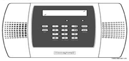
The keypad also features a built-in sounder, which will sound during alarms and troubles. The keypad also "beeps" during certain system functions, such as during entry/exit delay times, in Chime mede, and when depressing any of the keys (to acknowledge the key press). In addition, a built-in speaker announces system status.
