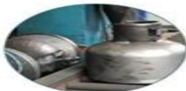
welding of guard ring
