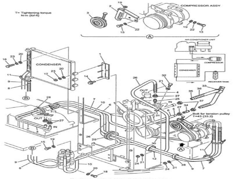
Fig. 25-2 Installing air conditioner and heater
