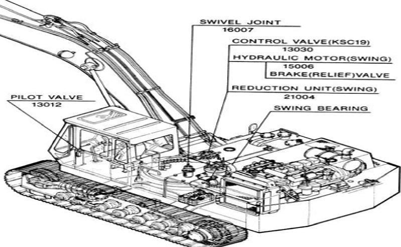
The swing system is designed to freely rotate or stop the upper frame on the lower frame; it comprises, in addition to the control valve, the hydraulic motor used for converting hydraulic energy into rotational force, reduction unit, bearings, swivel joints, etc.
