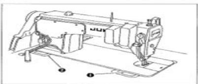
Fit hinge into the opening in the machine bed, and fit the machine head to table rubber hinge before placing the machine head on cushions on the four corners.
