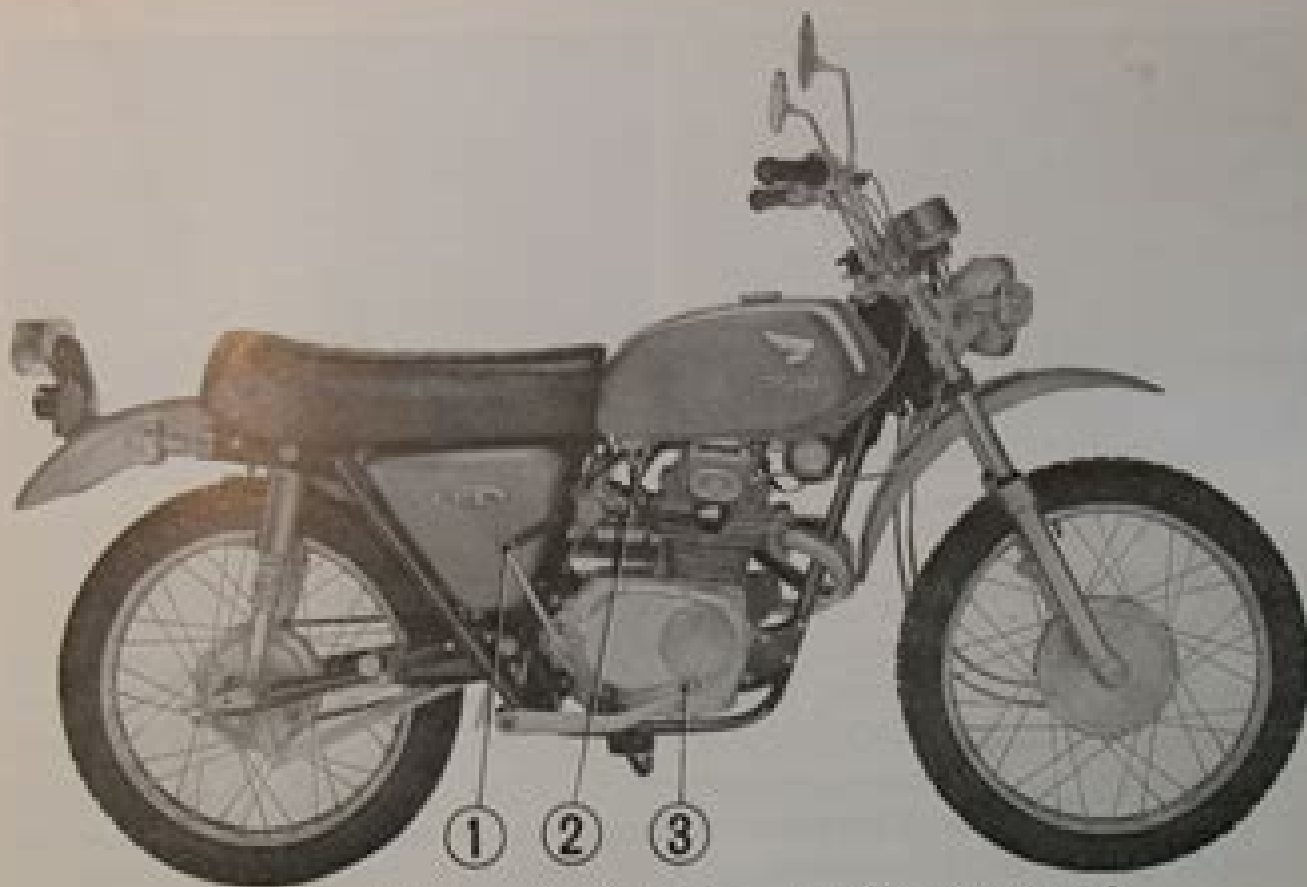
① Kick starter ② Fuel cock ③ Rear break pedal
