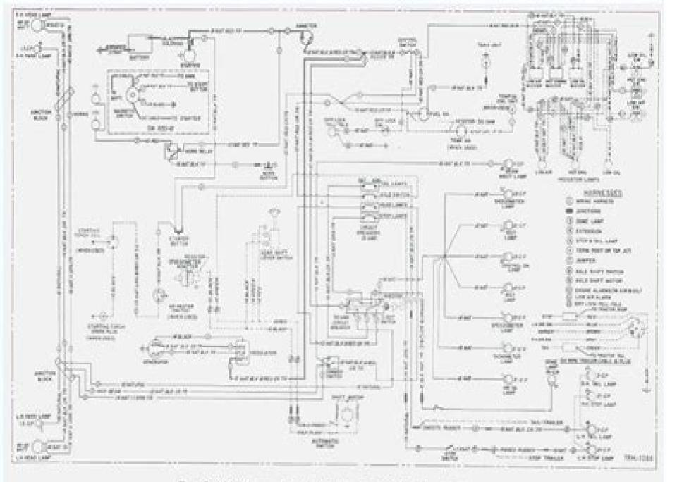
Figure 3 -- Wiring Diagram -- Early Diesel Models -- Series D620-47 Through D660-47
