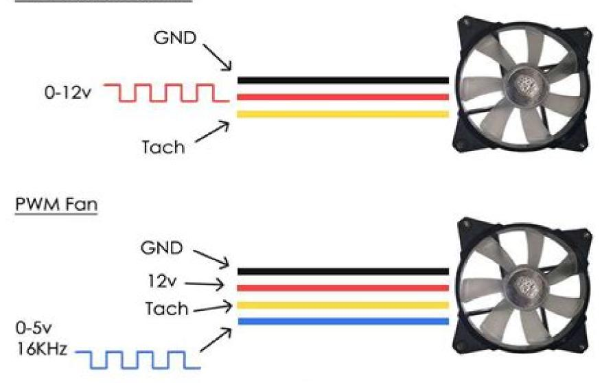
All you need to control the speed of a PWM fan is a 5v square wave at 16KHz.
