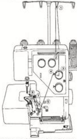
Place the spool of thread on the spool pin second from the right.
